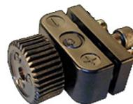
The unique design of these binding posts allows the use of a strong, hard material for the threads that provide the pressure on the connection, while at the same time using optimal electrical connections (which require a softer metal). By separating the mechanical and the electrical systems within the connector, both can be properly optimized.
