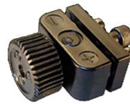
The unique design of these binding posts allows the use of a strong, hard material for the threads that provide the pressure on the connection, while at the same time using optimal electrical connections (which require a softer metal). By separating the mechanical and the electrical systems within the connector, both can be properly optimized.
